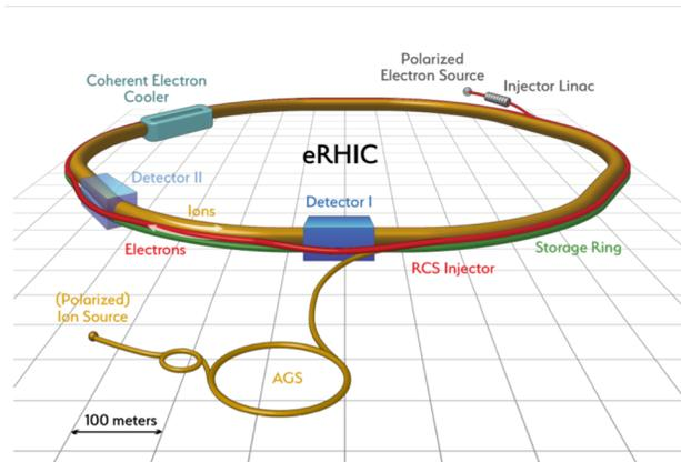
Figure 1: Conceptual layout of eRHIC.
