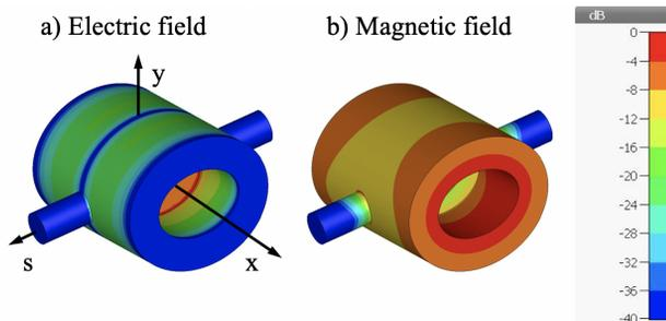
Figure 2: Electromagnetic field distribution for fundamental (crabbing) mode of the 200 MHz elliptical-section DQW cavity generated with CST Microwave Studio [14].
