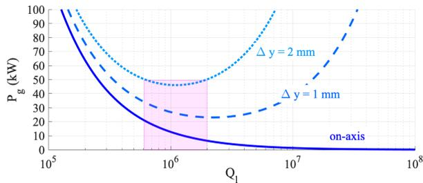
Figure 3: Generator power required by a 200 MHz crab cavity with  $(R/Q)_\perp = 610 \Omega$  and  $Q_l = 2 \times 10^6$  for delivery of 5.5 MV deflecting voltage to 1 A average current beam. Power requirement below 50 kW in framed region.
