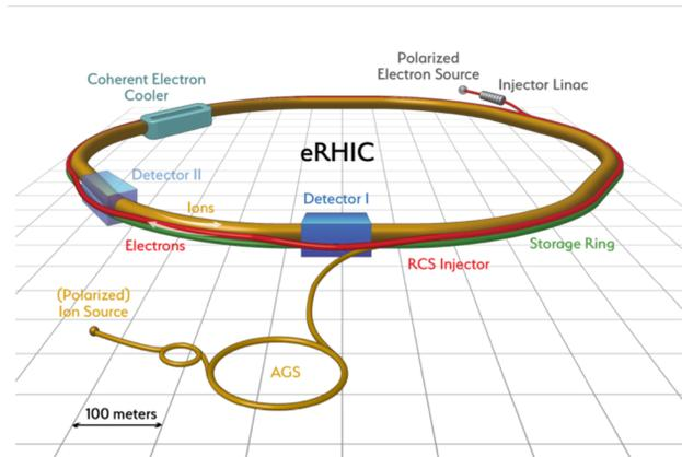
Figure 1: Conceptual layout of eRHIC.
