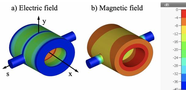
Figure 2: Electromagnetic field distribution for fundamental (crabbing) mode of the 200 MHz elliptical-section DQW cavity generated with CST Microwave Studio [14].
