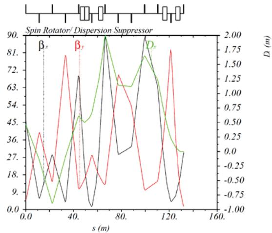
Figure 5: This is an overview of the spin rotator/dispersion suppressor section in the HEB.
