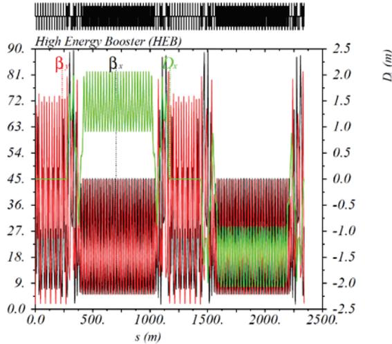
Figure 3: The optics functions of the HEB.
