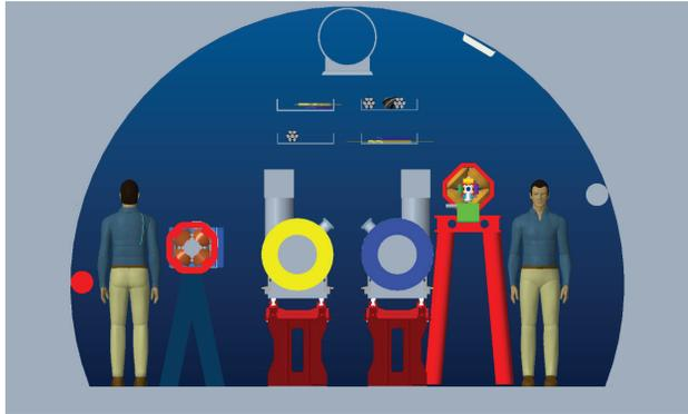
Figure 1: eRHIC tunnel cross section with the electron storage ring in the same plane as the two existing RHIC ion rings, and the injector synchrotron above.
