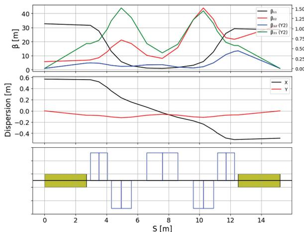
Figure 3: Rotator solenoid section with five quadrupoles in-between solenoid segments for coupling compensation.
