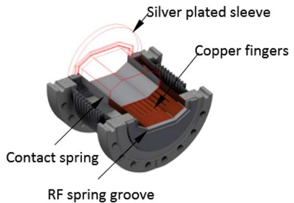
Figure 6: NSLS-II bellows with RF fingers on the outside.
