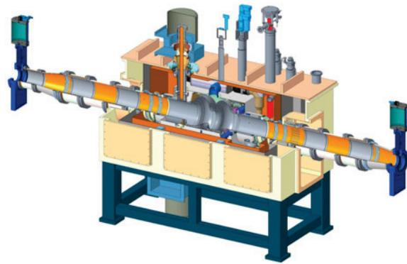
Figure 5: 591 MHz RF cavity with fundamental power couplers and higher order mode dampers.
