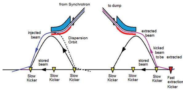
Figure 4: Schematic view of the off-energy injection and extraction scheme.
