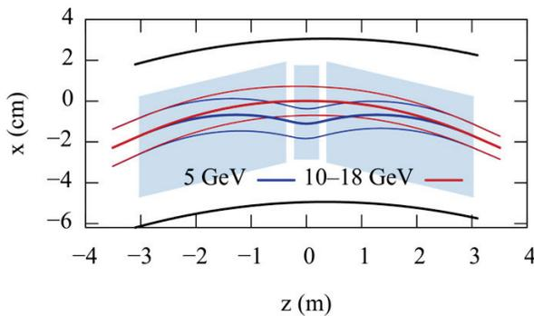
Figure 2: Schematic layout of a super-bend dipole.
