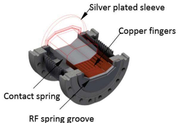
Figure 6: NSLS-II bellows with RF fingers on the outside.
