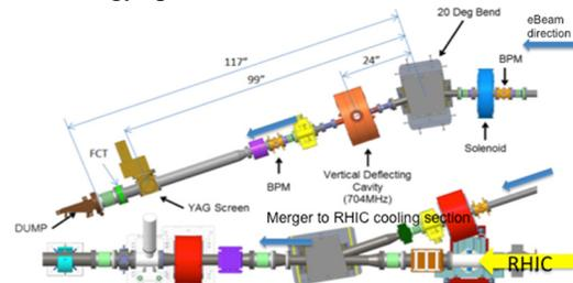
Figure 3: RF diagnostic line layout.
