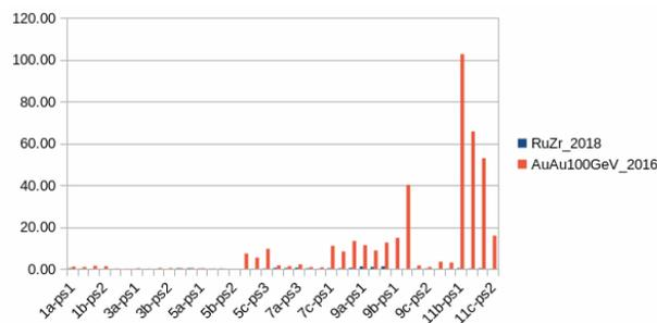
Figure 4: Diagnostic memory upsets per day by alcove for Run-16 (Au+Au) and Run-18 (Ru+Ru/Zr+Zr).
