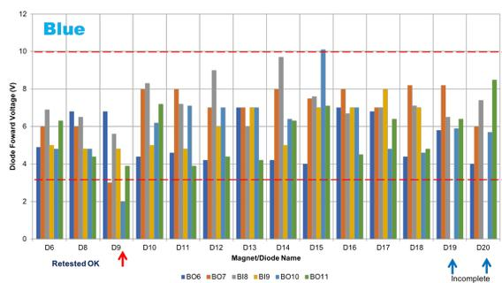
Figure 3: Measured forward bias voltage of Blue dipole quench protection diodes. Only one diode, at the location of a short dipole, was found with out of specification.
