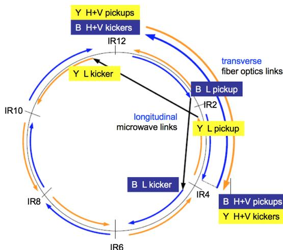
Figure 1: Present layout of the RHIC stochastic cooling systems.
