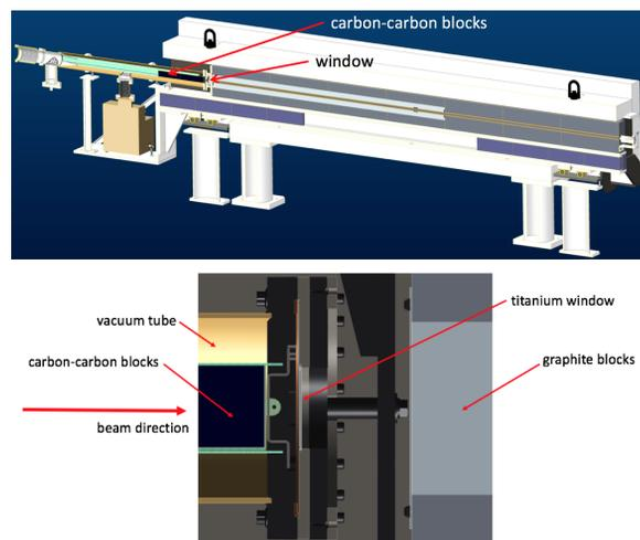
Figure 2: RHIC beam dump (top) and window detail (bottom) after the 2014 upgrade.
