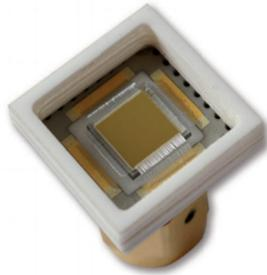
Figure 1: Photograph of diamond Knopf-detector, used for tests at CERN.
