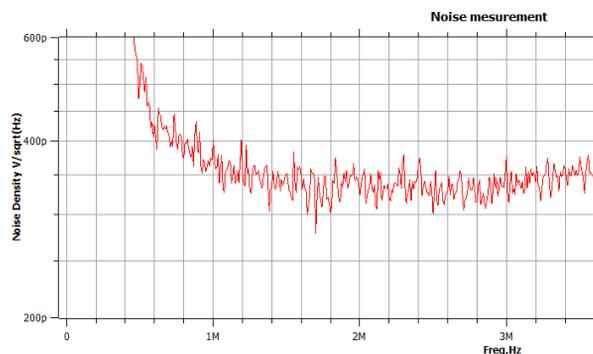
Figure 5: Noise measurements of cryogenic detector as function of frequency.
