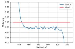
Figure 7: Three-dimensional local magnetic field gradient  $k_{local 3D}$  as a function of radius.
