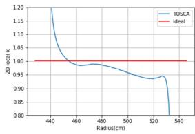
Figure 6: Two-dimensional local magnetic field gradient  $k_{local\ 2D}$  as a function of radius at the center of the F pole.
