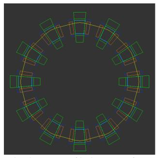
Figure 2: Arrangement of the electromagnets of PPR.
