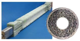
Figure 3: a) FRP support beam, formed by assembling 'window-frame' segments of G-11 FRP onto the 316SS beam tube, vacuum-impregnating the assembly, and precision-machining the half-round channels that position each CIC turn; b) cross-section photo of 2-layer NbTi CIC.
