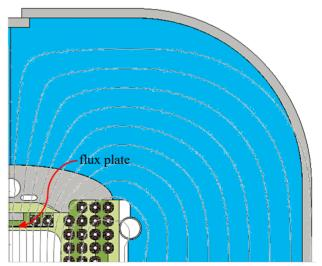
Figure 5: Quadrant cross-section of the 6 T CIC dipole: green – G-11 structure elements, blue and gray – steel flux return. Note the steel flux plate.
