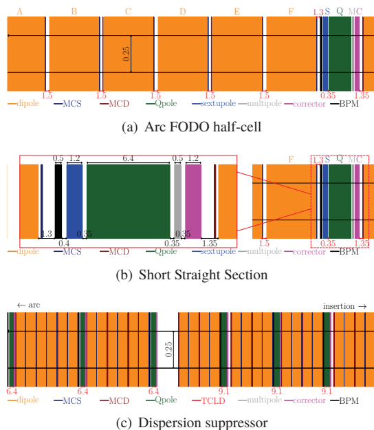
Figure 2: Layout of the arc FODO half-cell, SSS, and DIS.
