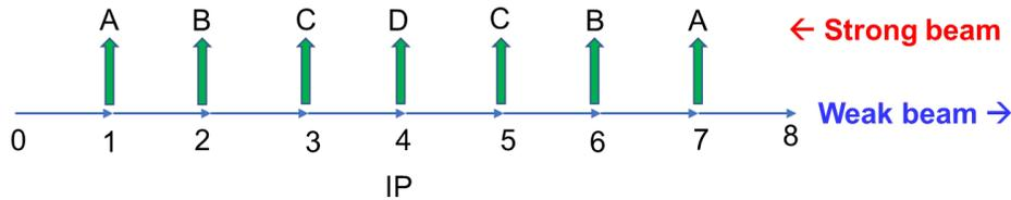
Figure 3: Schematic of the beam-beam interactions labelled A through D either side of the IP at parasitic interaction points labelled 1 through 8. In reality there are many more such long-range interactions as bunches pass one another.
