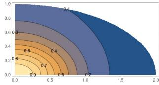
Figure 6: Electric field slope Ey(x,y)/y for N=10.
