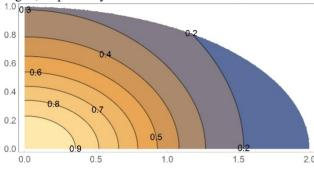
Figure 3: Electric field slope Ex(x,y)/x for N=6.
