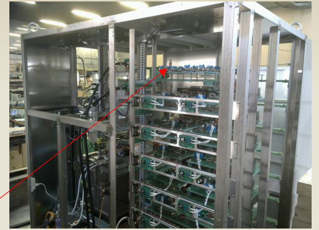
Ultrafast recovery diode (CKE CKF12P100D1D) 1.2 kV, T_{rr} \sim 135 ns
