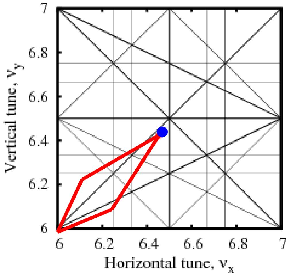
RCS tune diagram and the operating point at injection.
