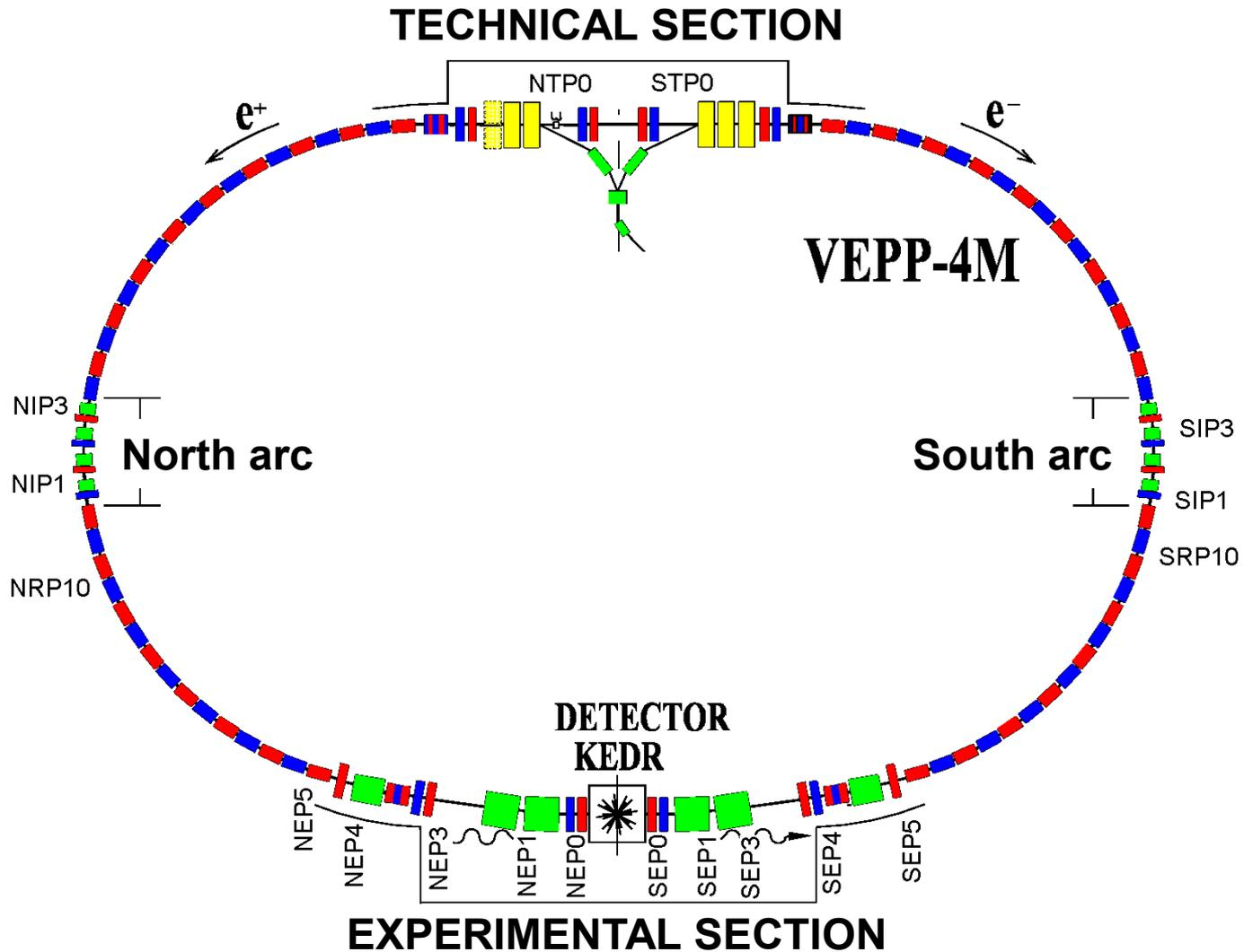
Figure shows positions of BPMs near four interaction points (IPs).
