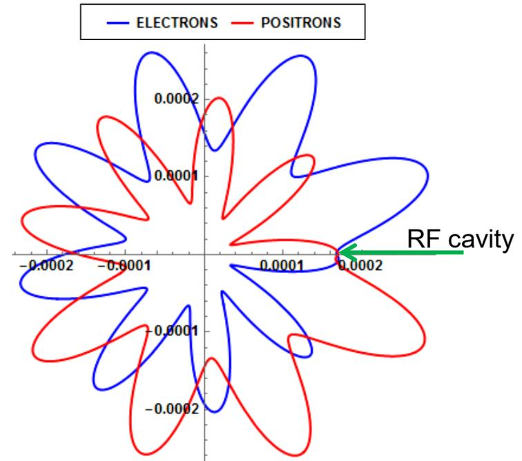
The  $e^-$  and  $e^+$  orbits in the azimuthally homogeneous model
