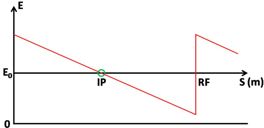
Saw-Tooth effect in particle energy distribution along the storage ring
