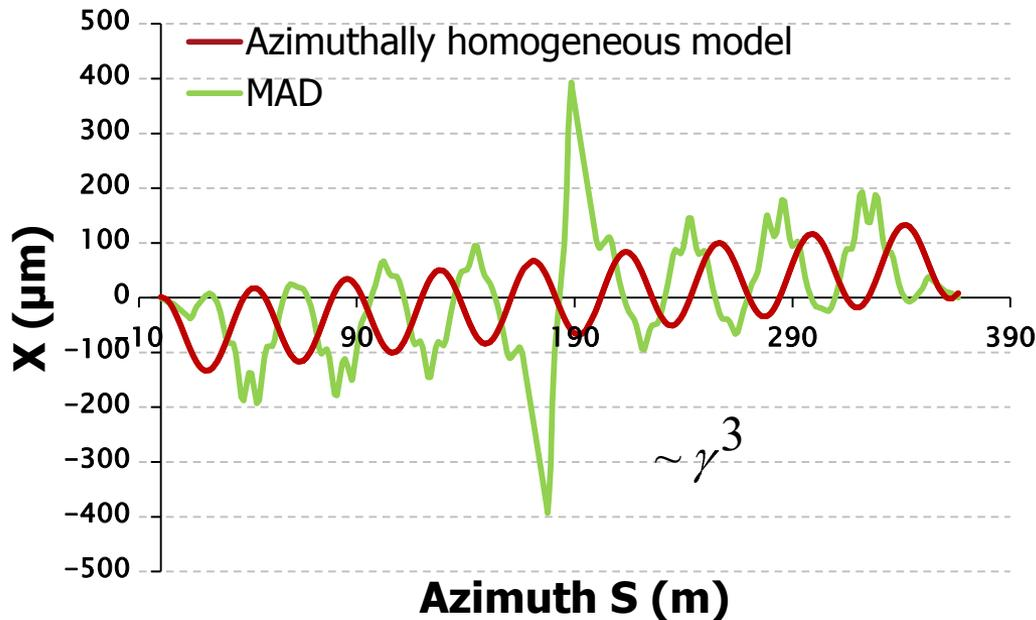
The maximum value of the difference between the electron and positron orbits is  $\sim 1 \text{ mm}$ .
