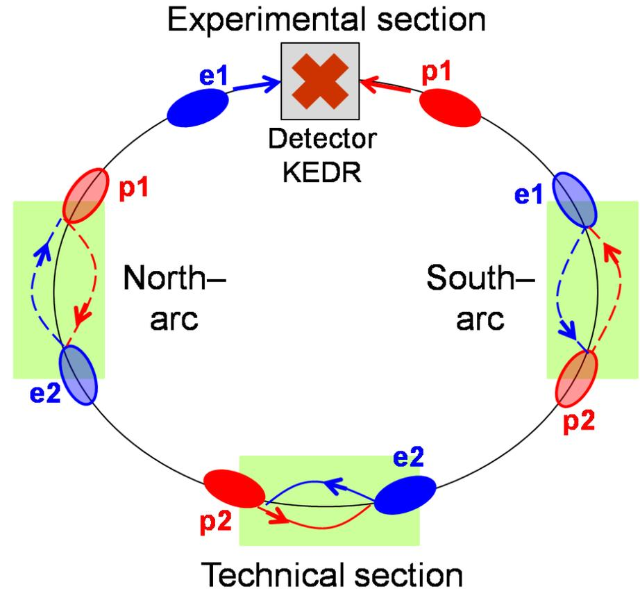
*Configurations of electron and positron bunches collision with a spatial quarter-revolution interval.*
