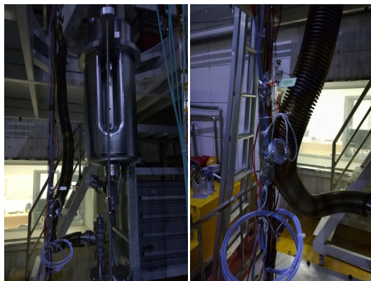
Figure 9: Position of second sound detector with HWR cavity.
