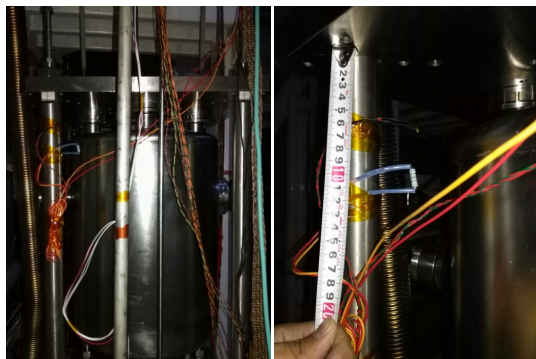
Figure 8: Position of second sound detector with QWR cavity.
