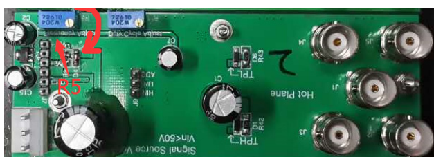
Figure 5: The rectangular pulse voltage source for the film resistor.
