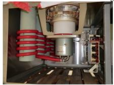
Figure 7: One of both tetrodes TH537 in anode down configuration. At the tube socket one sees the screen grid capacitor (500 nF) to ground unwanted RF currents. To the right there is the coupling capacitor and the contact tab to the cavity bus bar.
