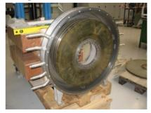
Figure 6: A pressure tank with four ring cores lined up.
