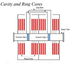
Figure 2: The arrangement for one cavity unit.
