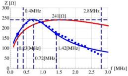
Figure 5: The resonance curve before (red) and after (blue) mounting the tetrode power amplifier to the cavity.
