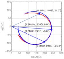
Figure 3: Measured (red)- and calculated (blue) impedance of one cavity half.
