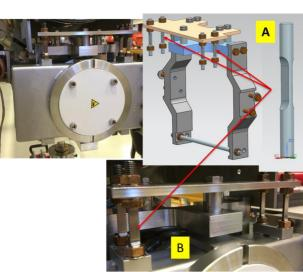
must maintain attribution to the author(s), title of the work, publisher, and DOI Figure 7: Tuner modification with flexible joints. (A) 3-D model of the cage to support gate valve. (B) Photo of the gate valve mounted with flexible rods.
