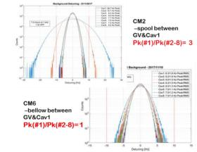
Figure 8: Microphonics measurements of cryomodule E F1.3-02 and cryomodule F1.3-06. F1.3-02 had no gate valve/cavity 1 modifications. F1.3-06 had the extended tuner arms and bellow between gate valve and cavity 1.
