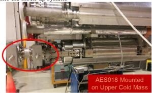
Figure 2: Picture of the mock-up for warm study of the proposed gate valve/cavity#1 modifications.
