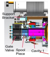
Figure 1: Picture of the "standard" interface between cavity#1 and gate valve.
