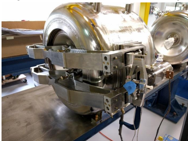
Figure 1: First article of the prototype SSR1 tuner assembled on a cavity.
