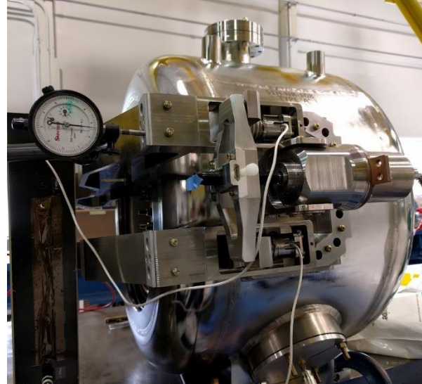
Figure 4: Stiffness measurement as measured with relative tuner component motion.
