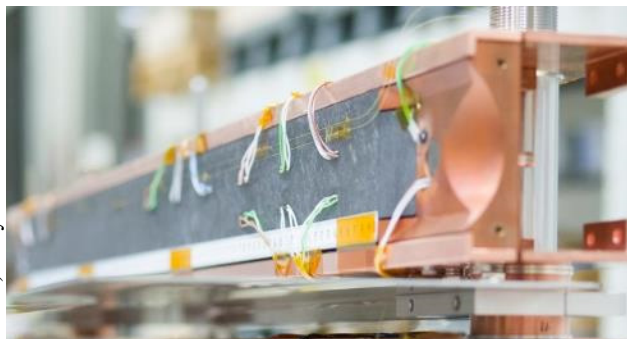
Figure 3: Collimator jaw equipped with resistive strain gauges and distributed optical fiber sensors over its length.
