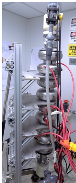
Figure 2: The 9-cell cavity on the 9-cell scale Bipolar-EP system at Faraday Technology.
