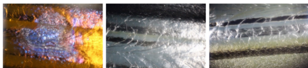
Figure 3: Optical inspection images of the equator weld seam post Bipolar EP with 4% (left), 9% (middle), and 11% (right) of H 2 SO 4 .
