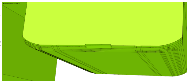
Figure 3: End chamfer of the D2 magnet.
