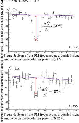
Figure 5: Scan of the PM frequency at a doubled signal amplitude on the depolarizer plates of 3.1 V.
