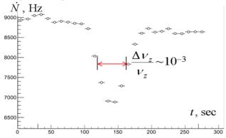
Figure 2: Typical behavior of the Touschek counters over time during scanning the PM frequency near the vertical betatron resonance.
