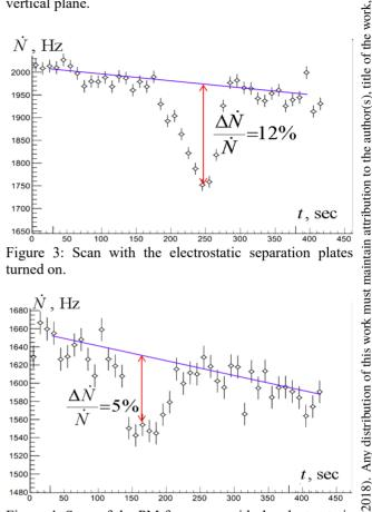
Figure 4: Scan of the PM frequency with the electrostatic separating plates turned off and a vertical displacement of the closed orbit down of 0.82 mm due to the TZ bump.
