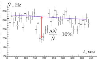
Figure 6: Scan of the PM frequency at a doubled signal amplitude on the depolarizer plates of 0.52 V.
