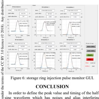
Figure 6: storage ring injection pulse monitor GUI.
