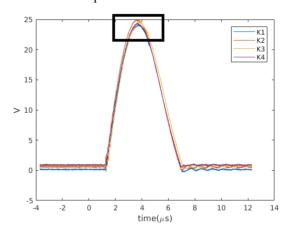
Figure 2: The aligned pulses of four units kicker power supplies.
