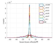
work Figure 4: Residual beam-beam offset with feedback for different relative luminosity precisions.
