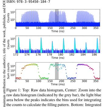
Figure 1: Top: Raw data histogram, Center: Zoom into the raw data histogram (indicated by the grey bar), the light blue area below the peaks indicates the bins used for integrating the counts to calculate the filling pattern. Bottom: Integrated counts for the 184 RF buckets.
