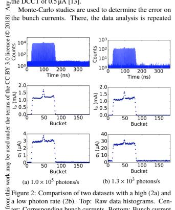
Content from a low photon rate (2b). Top: Raw data histograms. Center: Corresponding bunch currents. Bottom: Bunch current errors.
