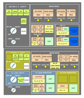
Figure 8: Image example of the modified (top) and old version (bottom) operation control panel.
