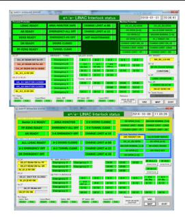
Figure 4: Image example of Interlock status display after system update (top) and before system update (bottom).
