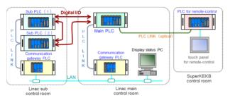
Figure 3: Schematic layout of safety management interlock system of Linac.
