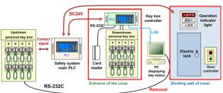
Figure 6: Schematic layout of the updated personal key management system to enter the accelerator room.
