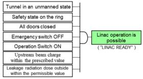
Figure 2: Linac operation conditions taking human safety into consideration on radiation.
