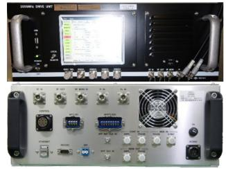
Figure 4: Front/rear panel of LLRF control unit.
