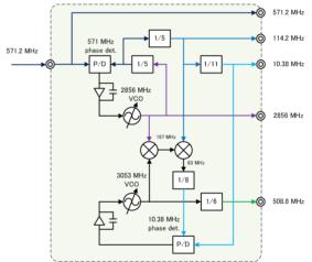
Figure 4: Block diagram of the frequency multiplier/ divider.
