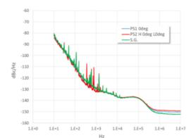
Figure 3: Phase noise distribution of the signal from the first I/Q modulator (blue), the second I/Q modulator (red), þ and signal generator (green). mav
