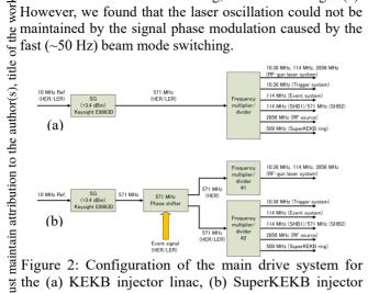
the (a linac. the (a) KEKB injector linac, (b) SuperKEKB injector
