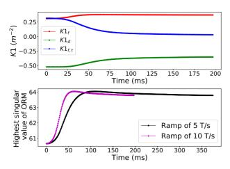
Figure 1: Top: Triplet to doublet quadrupole transition over the ramp.  $K1_f$ ,  $K1_d$  and  $K1_{f,t}$  are the normalized strengths of the doublet focusing, doublet defocusing and triplet focusing quadrupole families of SIS18, respectively. Bottom: Variation of vertical ORM over ramp.
