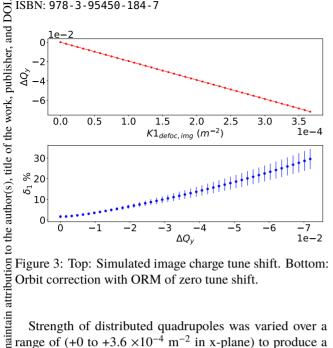
Figure 3: Top: Simulated image charge tune shift. Bottom: Orbit correction with ORM of zero tune shift.
