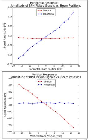
Figure 3: The difference in signal amplitudes of the opposite electrodes as a function of the horizontal (vertical) beam position.
