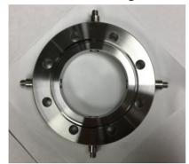
Figure 1: The in-flange simplified button-type BPM pickup device.
