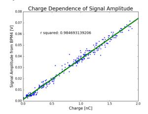
of the CC BY 3.0 licence (© 2018). Any distribution of this work must maintain attribution to the Figure 2: The combined signal strength of four electrodes terms of the in-flange pickup device, as a function of charge.
