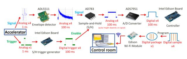
Figure 4: The mockup wireless BPM system using the COTS Intel Edison board.
