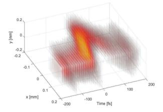
Figure 3: Tracked particle distribution at the screen with the TDS off (top) and reconstructed beam distribution using 16 streaking angles (bottom). The beam is divided into 10 fs temporal slices in accordance with the calculated resolution. The colour map illustrates the charge density profile and has been normalized to the maximum intensity in each plot.
