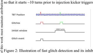
Figure 2: Illustration of fast glitch detection and its inhibit uo functionality. A 1000 turns inhibit window masks predictable disturbance like the injection transient.
