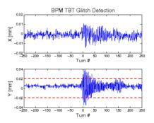
Figure 3: BPM TBT data captured with the fast glitch technique, X/Y are horizontal/vertical positions. A global trigger event was distributed at turn #0 where vertical position went outside the threshold of 20µm (red dashed lines).
