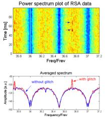
Figure 5: (top) FFT spectrum captured at fast ion glitches, around 50ms and 70ms where arrows point. (bottom) averaged spectrum with and w/o glitches.
