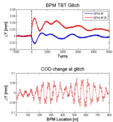
Figure 6: (top) TBT vertical position measured at the glitch showing orbit disturbance; (bottom) COD from synchronized BPM data around the ring.
