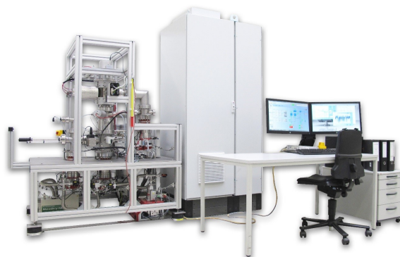
Figure 1: Overall view of the EBIS based low-energy fine-focus ion accelerator facility.
