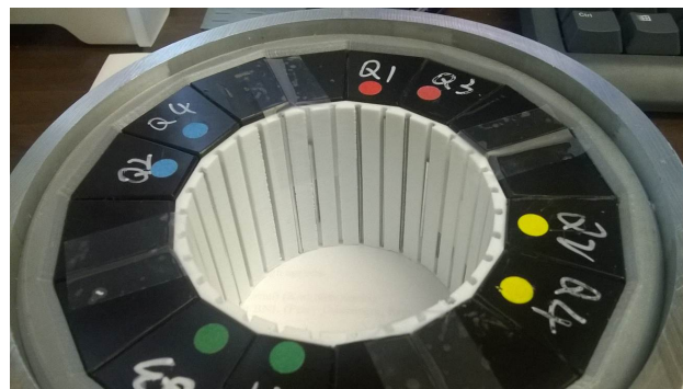
Figure 8: Halbach magnet using 3D printed mould and tuning insert containing iron wires.
