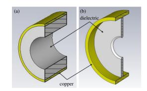
Figure 1: The section view of structures. (a) DLA; (b) A single cell of DDA.
