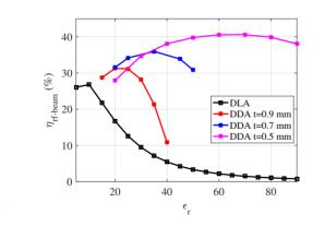
Figure 2:  $\eta_{rf-beam}$  as a function of the dielectric constant in different structures.
