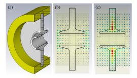
Figure 3: A single cell of the X-band DDA prototype. (a) Section view; (b) Electric field distribution; (c) Magnetic field distribution.
