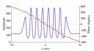
Figure 5: Distribution of the amplitude (blue) and the phase (red) of the on-axis electric field in the X-band DDA prototype. The power is fed from the left.
