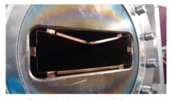
Figure 3: Collapsed RF-finger.
