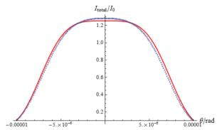
Figure 3: comparison of analytical results of angular flux density distribution for the 3<sup>rd</sup> order harmonic with the SPECTRA result. The dash line represent to the numerical results calculated by SPECTRA and the red line represent to the analytic result.
