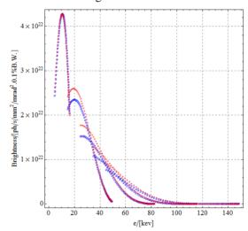
Figure 7: brilliance comparison of CPMU18 between the two different parameter schemes. The blue points refer to the scheme with emittance ex=34.2pm and energy spread  $\sigma \varepsilon = 0.106\%$  while the red points refer to the scheme with emittance  $\varepsilon x=40$ pm and energy spread  $\sigma \varepsilon=0.081\%$ . Any other parameters are the same as that in Fig. 6.
