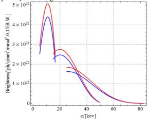
Figure 6: brilliance tune-curve of CPMU18. Where εx=34.2pm, βx=1.9m, εy=4pm, βy=2.2m and current I=0.2A. the remain parameters are the same as before. The red line represent to the brilliance of single undulator with the length doubled. The blue line is the brilliance of double undulator configuration.
