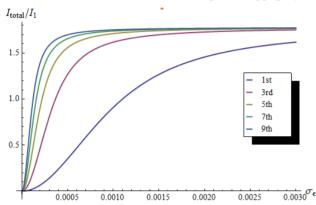
Figure 2: gain of on-axis angular flux density of different harmonics vary with energy spread on the condition of phase mismatched.(N=100 in both case)
