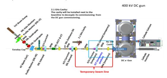
Figure 1: LEReC DC gun beam test layout. 2.1 GHz 3<sup>rd</sup> harmonic cavity (testing aside of DC gun test beam line) and 704MHz SRF cavities (shown as a blue box contour) will be installed in replacement of temporary beam line after gun end test is finished in fall of 2017.
