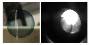
Figure 2: First cathode with scratch marks used in the DC gun test: (left) before installation, (right) cathode installed in the gun.
