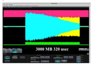
Figure 5: Gun FCT signal (yellow) and beam dump FCT signal (cyan) during 3000 Macro bunches operation.
