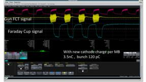
Figure 4: Charge per bunch reached minimum LEReC design requirement 120 pC. Cyan trace is beam dump faraday signal 4 macro bunches 30 of 704 MHz bunches each.
