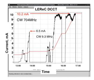
Figure 7: Beam current (black) measured by DCCT during CW operation with 9.4 MHz modulation up to 6.5 mA then ramp up to 10 mA 704MHz CW.
