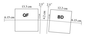
Figure 2: A synoptic of CBETA 5-degree bend, 44.4 cm long arc cell. QF is a pure quadrupole, focusing, BD is a combined function dipole, defocusing. The optical axis coincides with the bore axis in the Halbach magnets.
