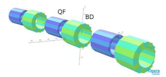
Figure 3: A 3-cell model in OPERA, with its quadrupoles QF, BD realized using the Halbach permanent magnet technology. The central (QF,BD) doublet field map can be used in the beam dynamics studies, or otherwise two independent field maps, one for QF and one for BD. The latter case offers flexibility, for instance it allows tuning fields independently, or moving the magnets relatively to one another.
