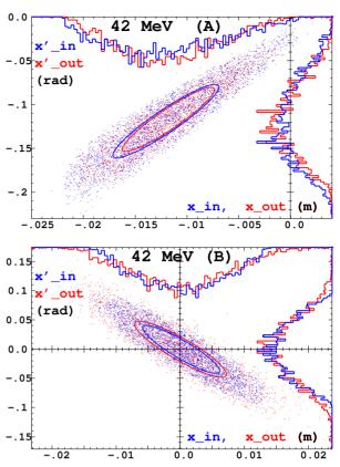
Figure 5: Horizontal (A) and vertical (B) initial (blue) and final (red) phase space coordinates, of the particles that make it through the 300-cell line, 42 MeV case. The blue and red ellipses are the *rms* matched ellipses, with surfaces respectively  $60\pi\mu$ m,  $110\pi\mu$ m.
