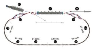
Figure 1: CBETA 150 MeV, 4-pass, 79 m circumference ERL, based on a 36 MeV superconducting linac and on a 107 cell NS-FFAG return loop using Halbach permanent magnet quadrupole technology. The return loop accepts the 4 recirculated energies in a single channel: 42, 78, 114 and 150 MeV.
