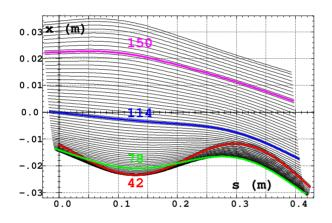
Figure 4: A scan in energy of periodic orbits across the 3-D full-cell map, 64 different energies over a 40-166 MeV range, the 4 design energies are thicker, colored curves. The 42 and 150 MeV orbit excursions reach  $\pm 2.33$  cm respectively, wrt QF bore axis. Nominal beam envelopes extend a fraction of a millimeter about these orbits.
