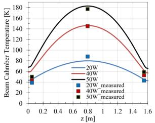
Figure 6: Beam vacuum chamber temperature along chamber length for three different heat dissipation levels. Solid curves are calculation, points are measured data.
