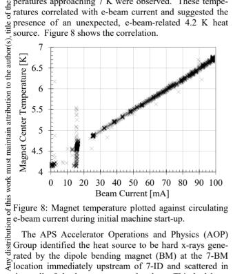
location immediately upstream of 7-ID and scattered in the wall of the beam vacuum chamber. This had been 8). flagged as a potential issue during device development 201 and installation planning. The solution involved an e-0 beam orbit correction through the BM. This orbit bump shifted the hard x-rays away from the vacuum chamber aperture, greatly reducing the heat load. This issue is 3.0] described in detail in [3].
