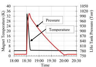
Figure 5: HSCU quench recovery. Magnet temperature spikes comparatively quickly while reservoir pressure decreases gradually over 1.5 hour.
