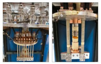
Figure 4: Cryocooler/corrector current lead package (left); cryocooler/main current lead package showing hightemperature superconductor (HTS) leads (right).
