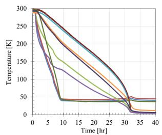
Figure 7: HSCU temperatures vs. time during cool-down. Thermal shield and beam vacuum chamber equilibrate rapidly compared to the 4 K elements due to the corresponding masses and available shield/4 K cooling powers.
