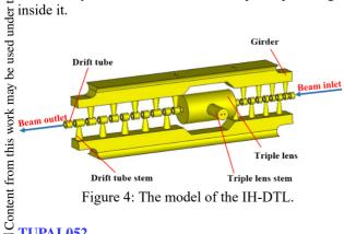
As shown in Table 2, the dimensions of the cavity have been optimized using CST MWS. Though the RF analysis, the cavity frequency and quality factor are 162.47 MHz and 14112, respectively. The frequency is close to the design frequency of 162.5 MHz, with a difference of only 0.018%. The power loss is estimated to be 85 kW.
