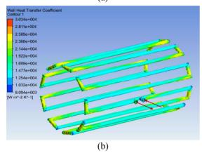
Figure 6: Heat transfer coefficients for the cooling system.(a) Girder water tank, stem and drift tube cooling channels.(b) Triplet lens cooling pipe.
