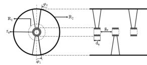
Figure 2: The schematic of a typical IH-DTL.
