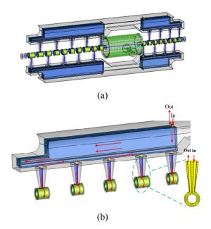
Figure 5: The cooling system. (a) Overview. (b) Enlarged view of cooling path.
