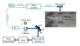
Figure 1: Schematic of fiber-optic strain sensor. SLD: superluminiscent laser diode, PD: photo-detector, FC: fiber coupler, M: mirror, BS: 50/50 beam splitter, PZT: piezoelectric transducer actuator, DAQ: data acquisition unit. Inset box: microscopic image of sensor head.
