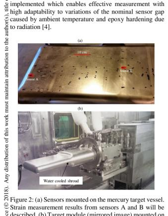
Strain measurement results from sensors A and B will be described. (b) Target module (mirrored image) mounted on target carriage in the target service bay. The target vessel is covered by water cooled shroud during operation.
