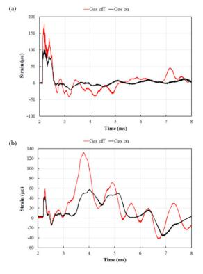
Figure 3: Strain waveforms measured with sensor A (a) and sensor B (b) at gas injection off and on. The proton beam power is 1.2 MW (equivalent) in both cases.
