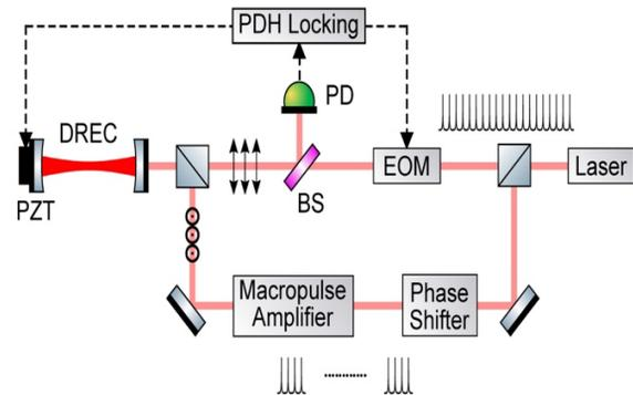
Figure 1. Schematic of double-resonant power enhancement cavity.
