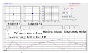
Figure 5:  $Ar^{9+}$  beam horizontal and vertical envelopes (red and blue lines) with the reconstructed beam  $\sigma$ -matrix just after the extraction electrode without space charge effects in TRACK simulation.
