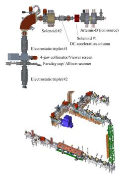
Figure 1: Layout of the FRIB Artemis-B ion source line (top) and FRIB Frontend line (bottom).
