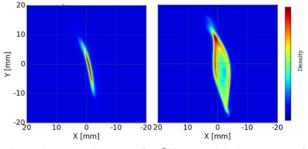
Figure 2: Screen images of Ar9+ beam with the current of 5  $\mu$ A (left), and 27  $\mu$ A (right) on each normalized color scale.
