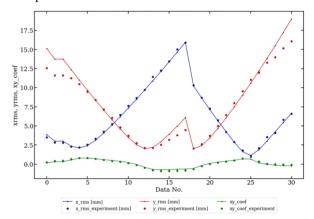
Figure 4: Electrostatic quad scanning result. Blue, red, and green dots denote horizontal and vertical beam size,  $\sqrt{\langle x^2 \rangle}$ ,  $\sqrt{\langle y^2 \rangle}$  in mm, and xy coupling coefficient is  $\langle xy \rangle/\sqrt{\langle x^2 \rangle}\sqrt{\langle y^2 \rangle}$ . Solid lines correspond to the fitting results.
