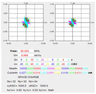
Figure 8: The transverse phase space distribution for Ar<sup>12+</sup> to Ar<sup>3+</sup> just before the first magnetic dipole in TRACK simulation.
