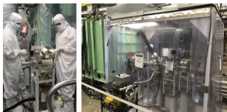
Figure 3: Left: Installation of a warm diagnostic box between cryomodules. Right: D-station.
