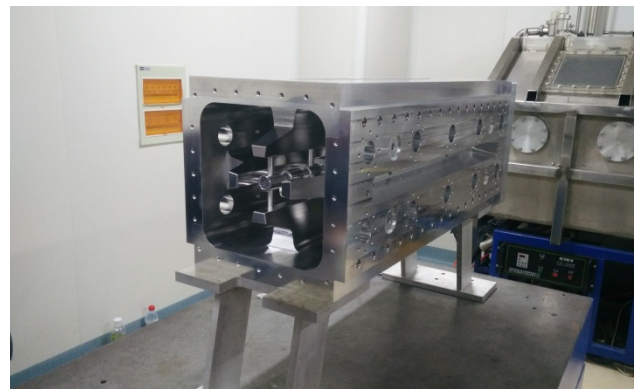
Figure 6: Hybrid RFQ prototype after assembly.
