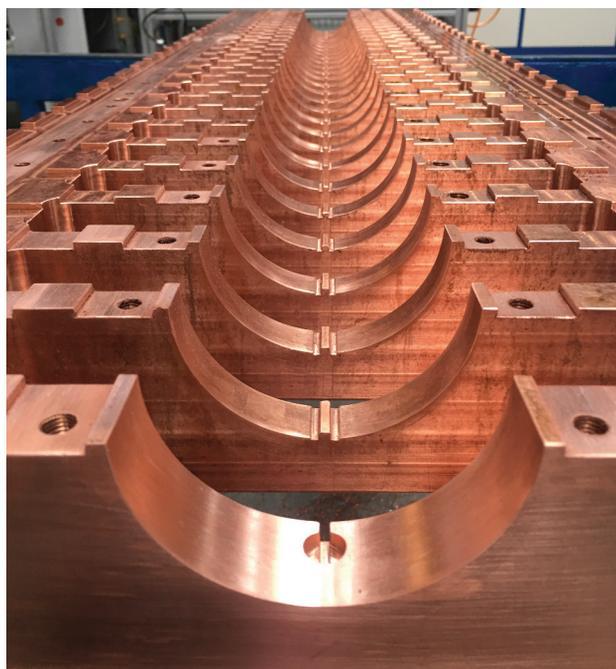
Figure 2: Lower half-ladder structure during the final finishing process.
