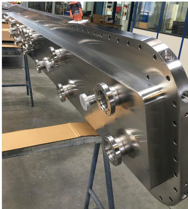
Figure 1: Upper tank shell of the Ladder RFQ after finishing of polishing ready for copper-plating.
