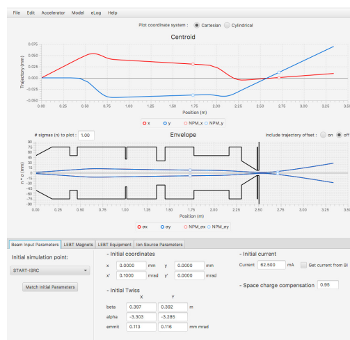
Figure 9: JavaFX GUI interface. The plots show the trajectory (top chart) and envelope (bottom chart) together with NPM readings.
