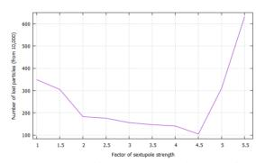
Figure 5: Number of lost particles as a function of the sextupole strength in Case 1. Units are chosen so that nominal sextupole strength corresponds to 1.
