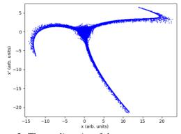
Figure 3: The nonlinearity of the resonance arms at high sextupole fields, if the tune is (i + 1/3). The phase space is shown just before the sextupole kick is applied.
