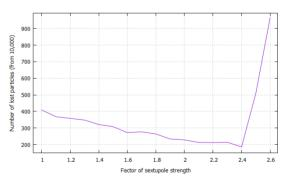
Figure 7: Number of lost particles as a function of the sextupole strength in Case 2. Units are chosen so that nominal sextupole strength corresponds to 1.
