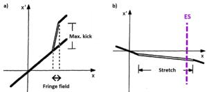
Figure 1: Effect of a massless septum kick applied to a linear particle distribution (a), and the reduced particle density hitting the ES wires (b). Figure modified from [9].
