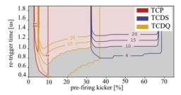
Figure 3: Number of bunches impacting in a critical transverse interval at the TCP, TCDS and TCDQ, depending on the relative number of pre-firing MKD and re-trigger time. Red: not acceptable; grey: acceptable.
