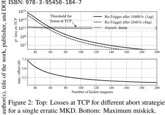
Figure 2: Top: Losses at TCP for different abort strategies for a single erratic MKD. Bottom: Maximum miskick.
